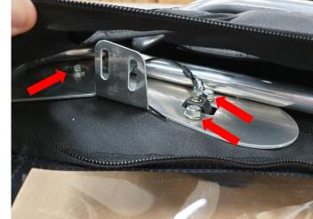
6) Install the rotary latch as shown using (2) 6mm bolts. Do not fully tighten at this time, so that the latch can still be moved for later adjustment.
