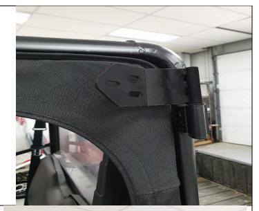
14) Press the upper door hinge against the door. Feel the fabric for the cutouts in the upper door frame plate. Make any adjustments necessary to both the door and the hinge for the best fit.
