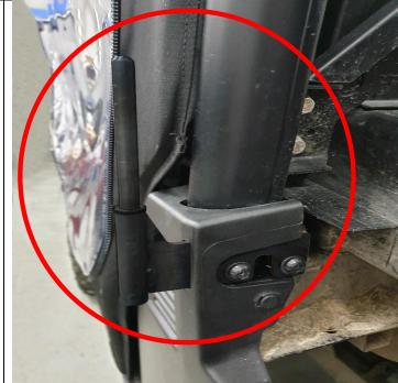
12) Set the door into the vehicle frame and latch the rotary latch onto the door striker. Position the door so that it is centered in vehicle frame. Adjust and tighten the rotary latch and striker if needed to help hold the front of the door closed and correctly positioned. Temporarily secure top rear of the door using a zip tie.
