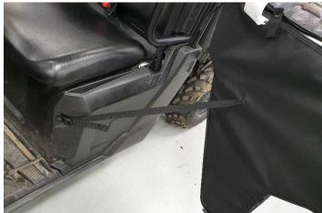
23) If any final adjustments are needed, loosen the door hinges slightly and adjust them so that door sits properly within the vehicle frame and opens and closes properly from both the inside and the outside of the vehicle.
