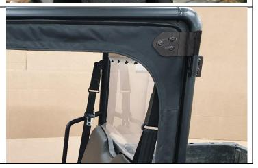
16) Install the lower door hinge onto the lower pin on top of the plastic washer. Be sure the hinge is oriented correctly.
