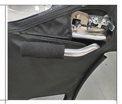
20) Slide shrink wrap tubing onto the cable portion of the 6mm eye end and cable installed in step (5). Install the cable to the latch.
