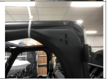
13) Install the upper door hinge onto the upper pin on top of the plastic washer. Be sure the hinge is oriented correctly.
