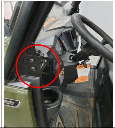
9) Install the upper vehicle hinge using (2) T40 Torx screws, (2) 8 mm flat washers and the nut plate removed in a previous step. Center the screws in the slots. Do not fully tighten the screws at this time. The hinge bracket should be secure, but still be able to move up and down for adjustment later.
