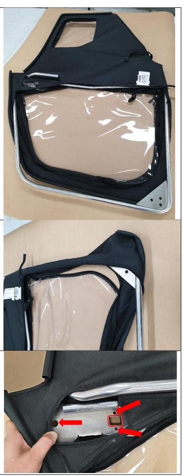
5) Install the outside door handle using (3) 6mm bolts and (1) 6mm fender washer. Only the front bolt will get a washer. Be sure that the handle sits flat against the plate and that the extended plastic boss seats into the front hole of the plate.
